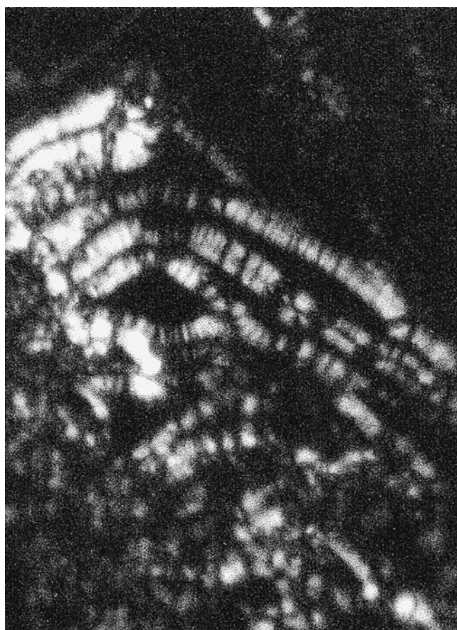
Fig. 5 Typical lamellar liquid structure observed through microscopic observation under polarized light observed for these transparent gels
